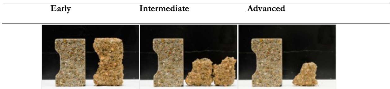
Figure 6. SCHN 158-treated samples are represented by the left concrete block. Pristine (untreated) samples are represented by the right concrete block.
