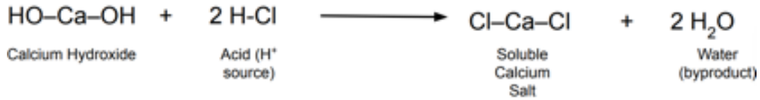
Figure 12. Chemical mechanism of acid attack on calcium hydroxide in cementitious materials. Acid reacts with alkaline cement phases to form soluble calcium salts, which leach from the structure and result in increased porosity and loss of structural integrity.
