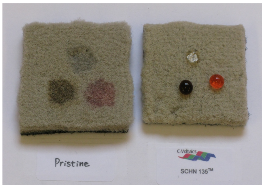
Figure 6: A test run using drops of water, juice, and grape soda on textiles. The left carpet is coated with pristine material, and the textile absorbs the liquids. On the right, the carpet repelled the polar liquids.
