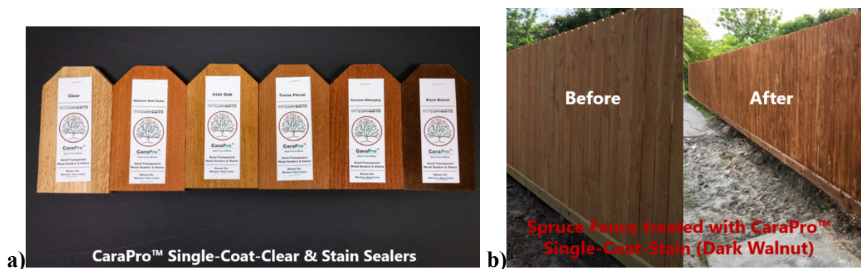
Fig. 10. SCHN application on wooden substrates. (a) Lab samples demonstrating aesthetic and functional pigmented sol-gel options. (b) Field application on an exterior spruce fence. The treatment regulates the supply of moisture and UV radiation, maintaining the construction below the threshold for biological colonization and structural decay.
